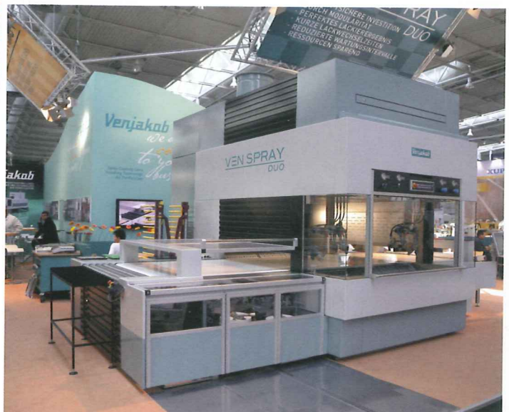
Below: Running at speeds of up to 20m/min, the newly designed Ven Spray Duo offers retroactive expandability. Latest developments include a redesigned fresh air supply, larger filters, precise air management in the spray cabin area, a redesigned belt cleaning and lacquer recovery system and fast changeover from one lacquer to another.
