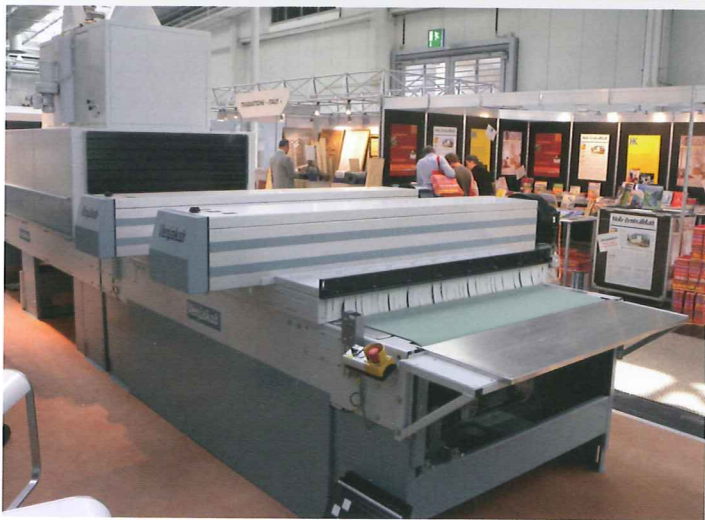
Above: The very latest Ven Dry UV enables surfaces and edges to be cured by means of a newly developed reflector. The IR portion of the light is greatly reduced, giving a cooler cure. This highly efficient system enables the curing of clear lacquers with only one lamp, thus providing significant energy savings.
